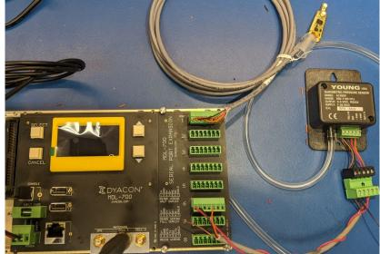
Here the TPH-1 is plugged into port 1, following the wiring diagram for RS485 halfduplex. The RM Young sensor is plugged into port 6 following the diagram for RS232 sensors. The ports used in this example are randomly chosen.
