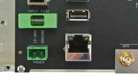
SMA antenna connectors for cell phone and GPS receiver.
