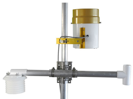
Image 2.2: Vertical Mast Mounting Position
