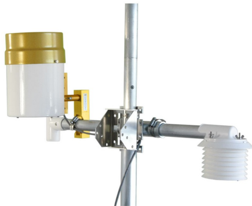
Image 2.1: Horizontal Pipe Mounting Position
