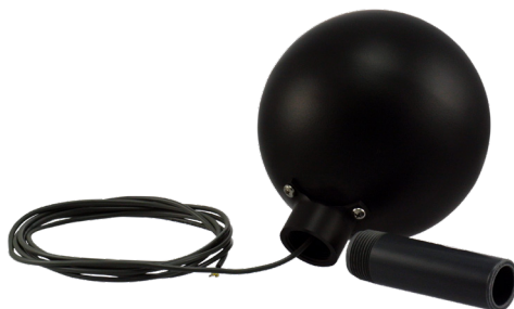
Image 1: Mounts to standard 1" NPT pipe
